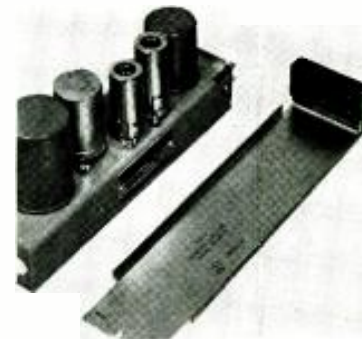
PLUG-IN PREAMP 3 which uses 5879 low-noise miniature tubes. It has an output level of +18 dbm, with less than 1/2% distortion, and a noise level of better than -120 dbm. It may be equipped with bridging volume control and meter connection.
